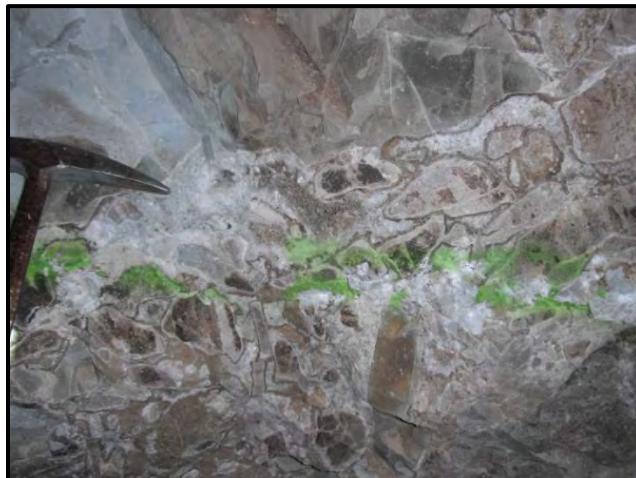
Photo 7-5: Breccia Style Mineralization Along Las Chispas Vein (Base of Las Chispas Gallery Near SilverCrest Sample 617179, 2.34 gpt Au and 343.5 gpt Ag, or 519 AgEq over 1.46 m)
