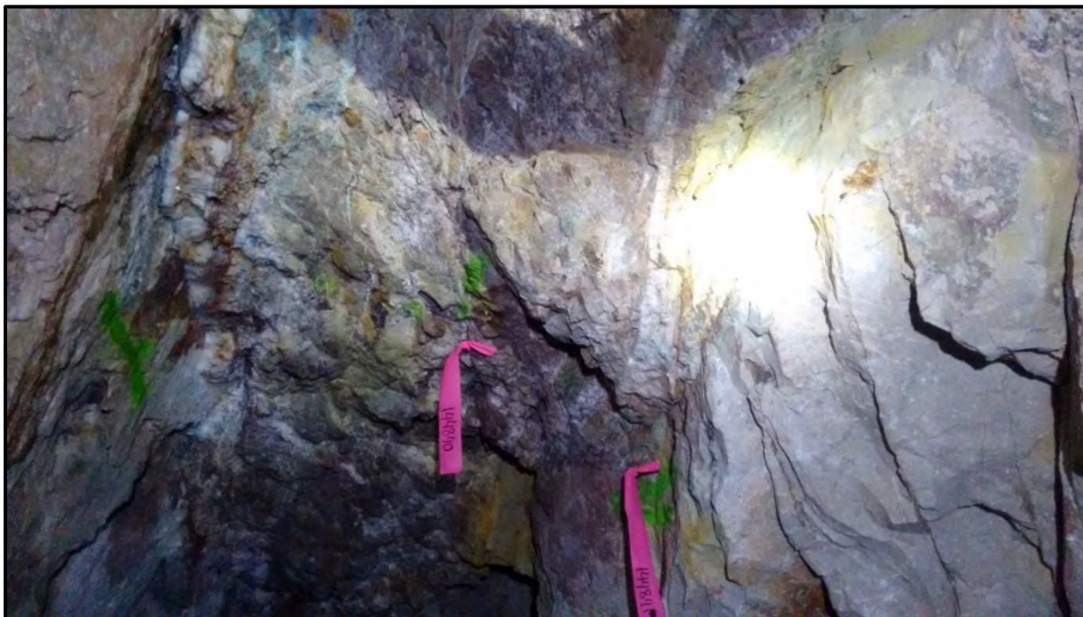
Photo 7-15: William Tell Underground Channel Sample No. 144840 Grading 13.4 gpt Au and 1,560 gpt Ag, or 2565 gpt AgEq
