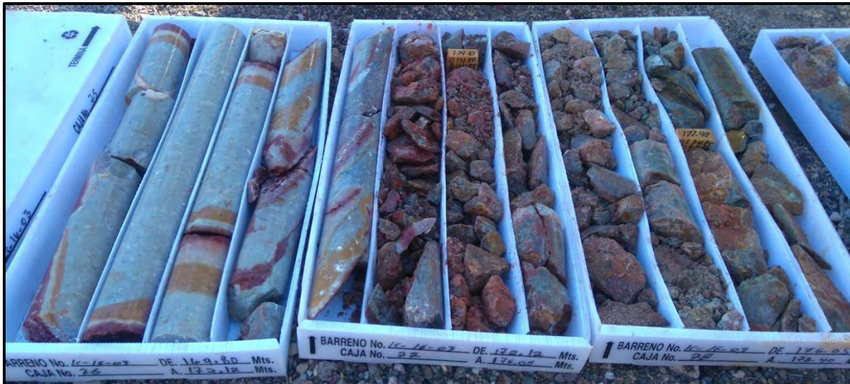
Photo 7-16: William Tell Vein, Drill Hole LC16-03; from 172 to 176 m, 4 m (1.5 m True Width) Grading 2.03 gpt Au and 683.0 gpt Ag, or 835 gpt AgEq
