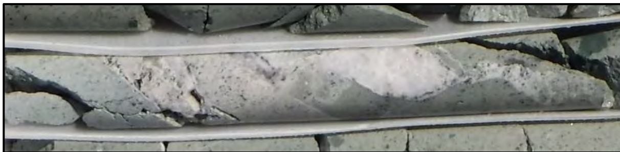
Photo 7-19: Drill Core, LC17-61 at La Blanquita, 116.0 to 116.55 m, 6.65 gpt Au and 1,445 gpt Ag, or 1,943 gpt AgEq in a Saccharoidal-Comb Quartz Vein
